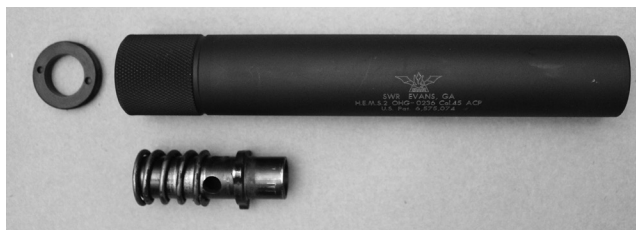
Figure 4.22 A functional suppressor manufactured by Southeast Weapons Research. It has been disassembled into its main components: the housing, recoil booster, and end cap. (Image from author's collection.)
